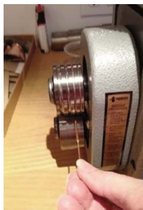
my rolling mill how I'd draw wire
